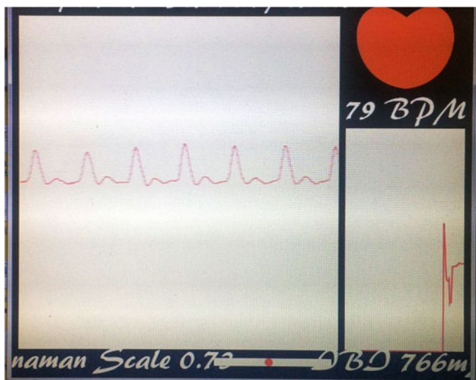
Fig. 6 Pulse output of the monitoring device
